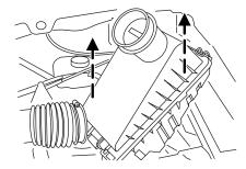
4. Release the two clamps that secure the cover to the air filter housing and place the cover aside.
